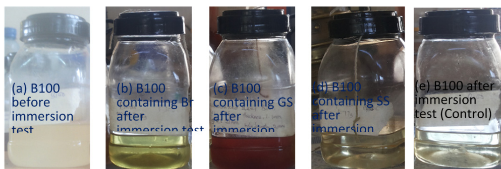
Fig. 6. Colour of Jatropha biodiesel (B100) (a) after production and after exposure to (b) brass (Br) (c) galvanized steel (GS) (d) stainless steel (SS), (e) without metal after eight weeks
