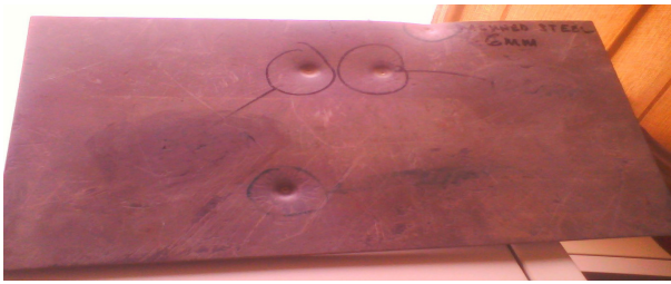
Figure 3: Frontal face- showing the plate's ballistic resistance against 0.30 calibres
