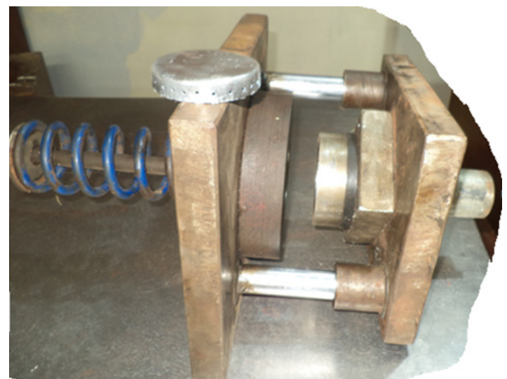
Fig. 3: Progressive and Combination Die with a sample of 2.0 mm Port Size Burner.
